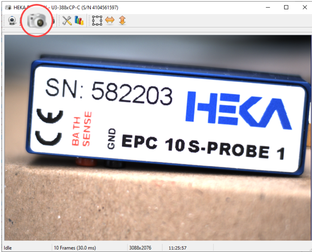
Figure 3.4: Snapshot button of the Image Window. The number of snapshots is provided at the lower border of the dialog.
