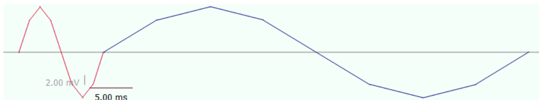
Figure 7.33: Example of a simple sine wave with separate frequency (2 Segments with 10 and 50 ms Duration, 10 mV Amplitude).
