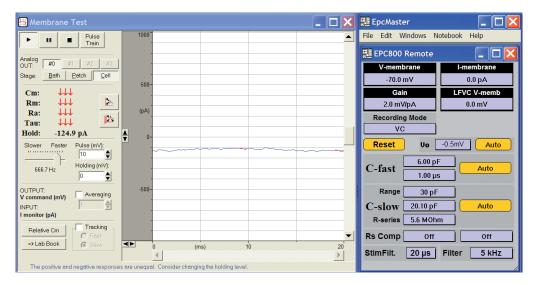
In this example, EPCMASTER is being used with a Digidata 1440A and Clampex software, the EPC 800 USB is now considered to be operated in remote mode.
